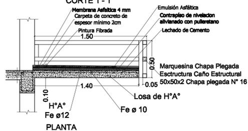
DETALLE LOSA H<sup>2</sup>A<sup>2</sup> (L1 a L6)
