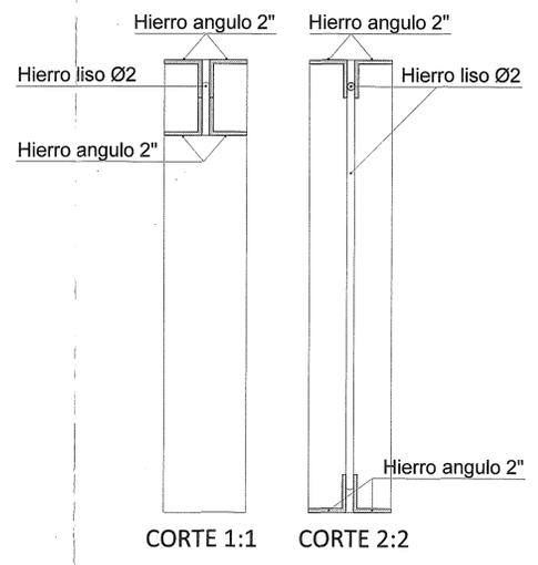
DETALLE DE VIGAS METÁLICAS "V1", "V2", "V3" y "V4"
