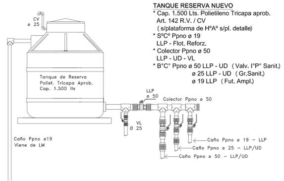
ESQUEMA TANQUE RESERVA Y COLECTOR
